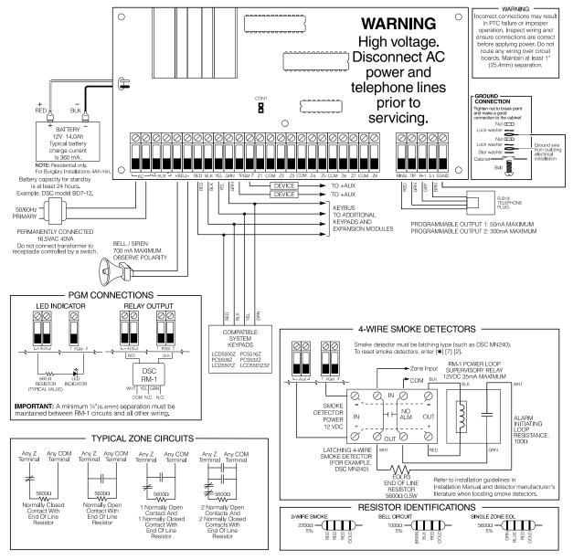
Temperature Range: 0°C-49°C (32°F-120°F) Maximum Humidity: 85% R.H. Refer to the Installation and Instruction Manuals for complete operating instructions. Compatible System Keypads: PC5508ZZ, PC5516Z, PC5532Z, LCD5500Z, LCD5501Z, LCD550
