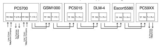
For example, if you are installing a PC5015 with a GSM1000 and a PC5928 Intercom module, connect the incoming line to the GSM1000, then from the GSM1000 to the PC5015, then from the PC5015 to the PC5928 Intercom and then from the PC5928 to the house telephones
