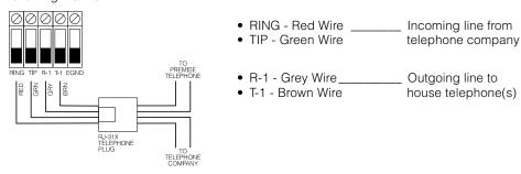
Connect the PC5015 and modules that use the telephone line(s) in the following order:
