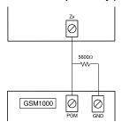
When using the GSM1000 cellular communicator, any main board zone may be configured for GSM1000 supervision. Program this zone as zone type [09], 24-Hour Supervisory in section [001].
